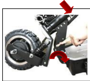
Step 2 Hold the pole by One hand; Press down the Red folding Lock by the other hand; Then fold the pole down
