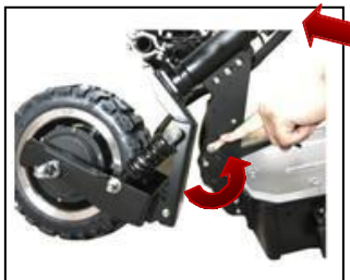
Step 1 Push down the folding Lock, and Push back the Pole At the same time
